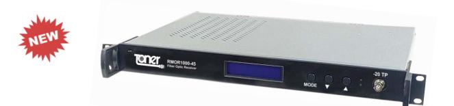
The RMOR1000-45 is a rackmount fiber optic receiver for receiving optical RF signals and distributing them in an RF system such as a CATV system or a PON network. This one-way node receives optical signals at 1310 - 1550 nm with a wide window of -8 to +2 dBm. The node has an output level of 45 dBmV while maintaining excellent distortion characters.
